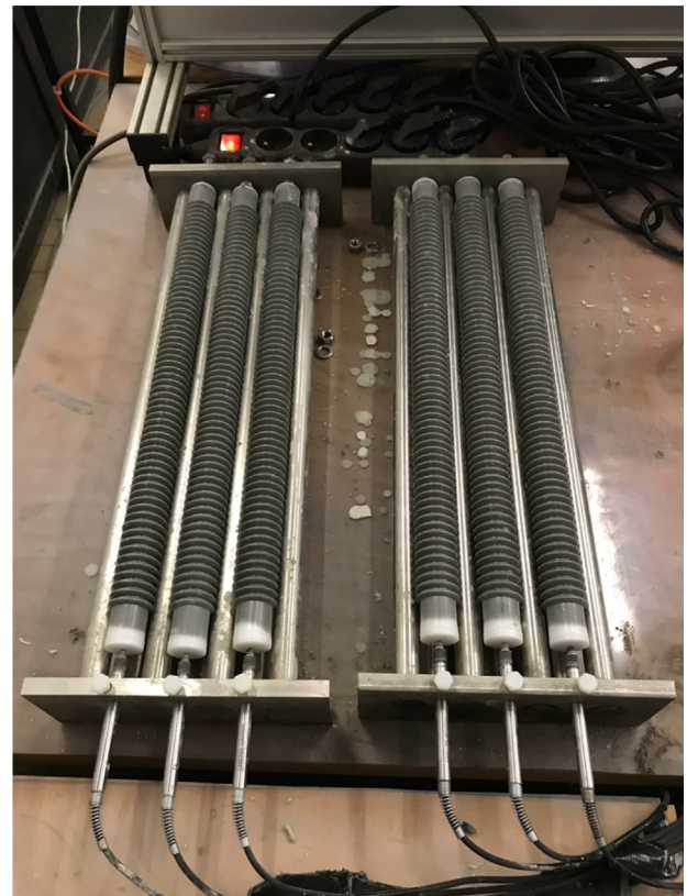
Fig. 1. Autogenous shrinkage test setup: corrugated tubes with LVDTs.
