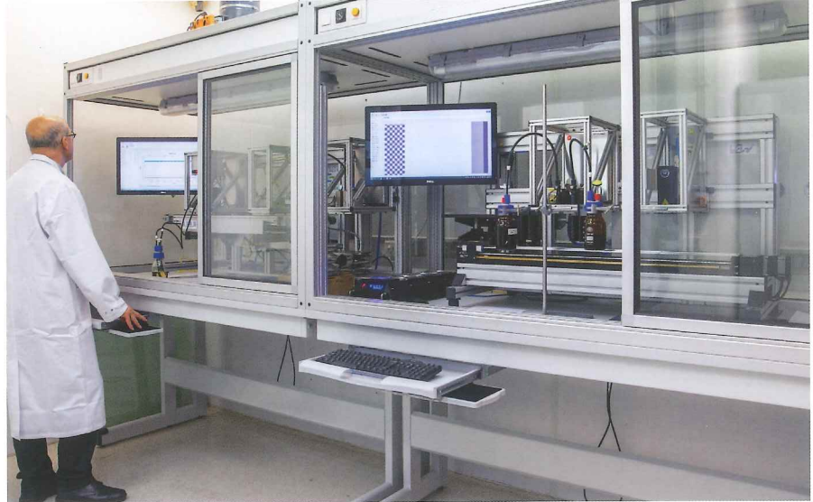
Figure 4: A modular 3D inkjet printing unit from VDW-Consulting. The printer is compatible with a range of industrial printheads such as Xaar, Toshiba-tec, Fuji Dimatix, Ricoh, Konica Minolta and Kyocera
