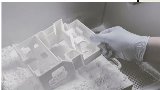
Thermoplastic Powder (PP, TPU, Nylon, PA,...) + melting/sintering
